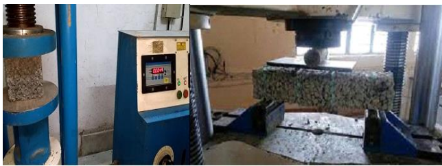
Figure 7 Compressive and flexure strength test
