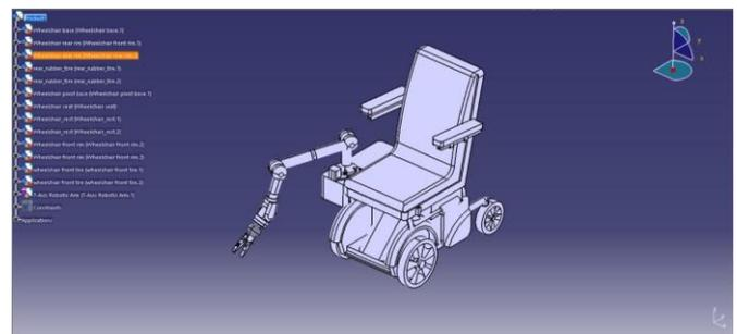
Fig 1. Wheelchair mounted mechanical arm design using CATIA V5R21
