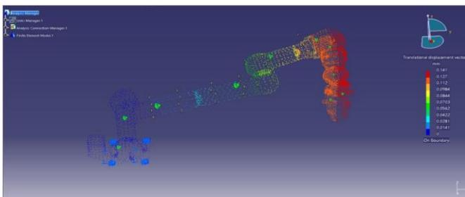
Fig. 5 Displacement of Mechanical Arm under practical weight (40N)
