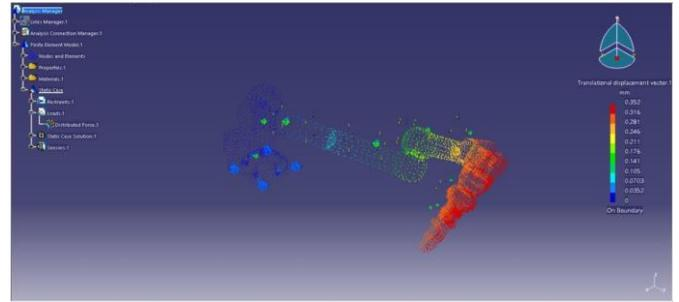
Fig. 6 Displacement of Mechanical Arm under load (100N)
