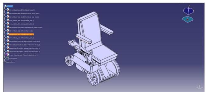
Fig. 2 Wheelchair with folded mechanical arm in CATIA V5R21
