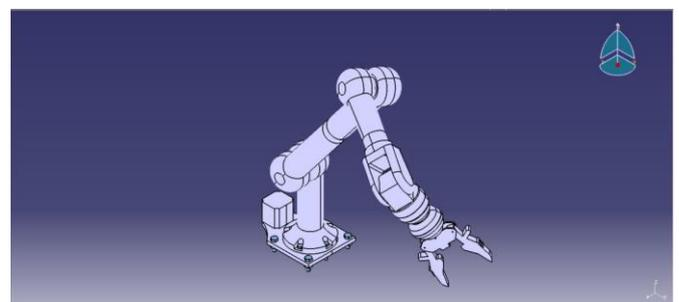
Fig. 2 Design of 7 Axis Mechanical Arm in CATIA V5R21
