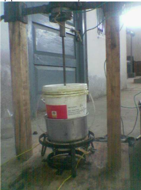
Fig. 2 Blender for mixing waster soya bean oil and catalyst.
