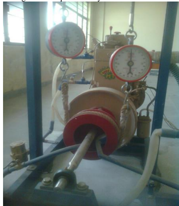
Fig. 1 Set-up For finding the brake power of C.I Engine (Rope Brake Dynamometer)
