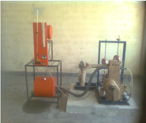
Fig. 4 Set-Up of Diesel Engine For Testing With Biodiesel.
