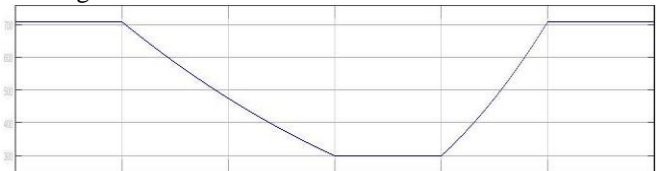
Fig. 9. Mechanical Power input to PMSG from Wind turbine
