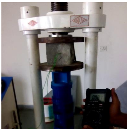
Figure 3. Testing Cube 1 under UTM
