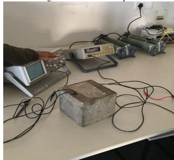
Figure 5. Damage analysis using Frequency Generator and CRO meter
