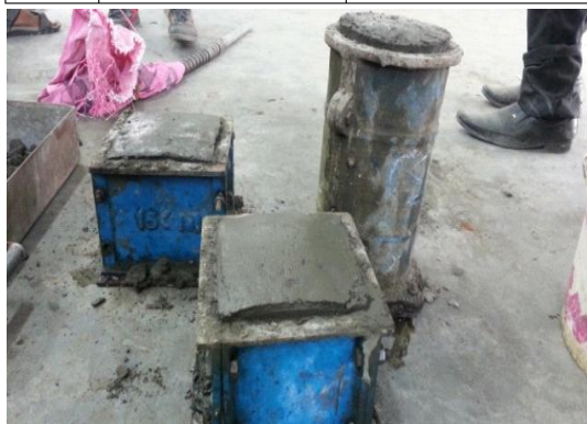
Fig6.Aluminium powder reaction on concrete
