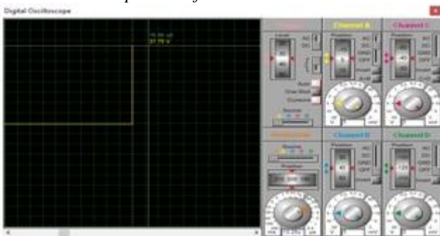
Figure 6. POSLC Simulation Output Wave Form The output voltage of open loop simulation of POSLLC. It has small overshoot and settles very fast.
