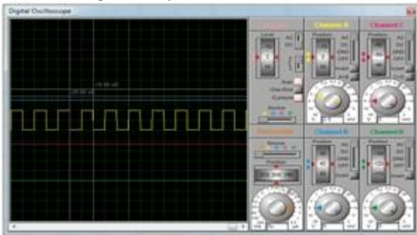
Figure 5. PWM MOSFET Switching Pulse Input Wave Form
