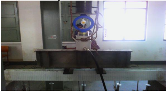
Fig 1: loading arrangement of beams
