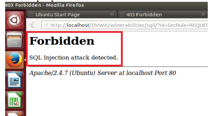
Figure 11: Prevention against SQLI scenario 2 We have also monitoring the audit log file of that scenario 2.
