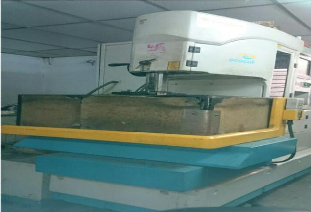
Figure 3.1- wire cut EDM,
