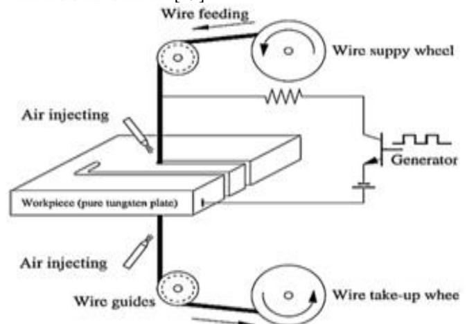
Fig. 1 the Basic Principle of WEDM Process
