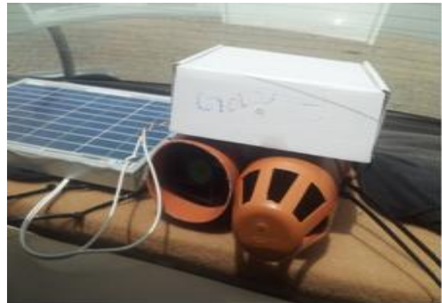
Fig.1. Existing solar ventilation system.
