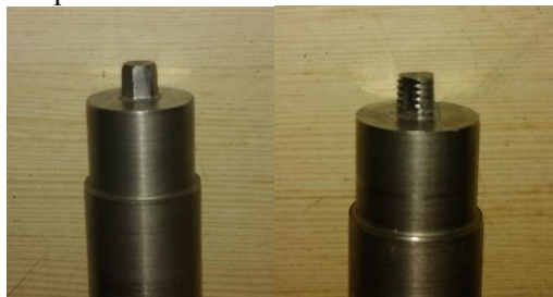
Figure 2 hexagonal and Triflute tool pin profile
