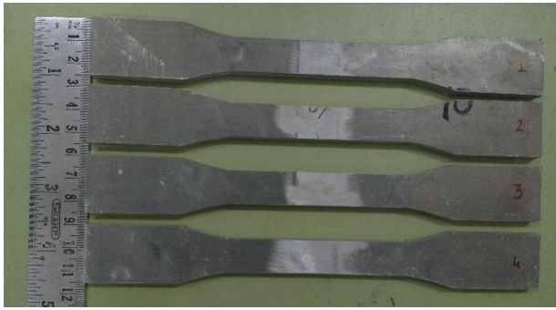
Figure 5 specimen for fatigue test as per ASTM E0466
