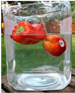
Figure 3, Buoyancy force was upward pushed the capsicum and apple body in glass.
