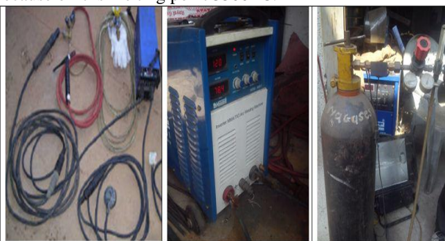
Fig. 3.2 TIG set up (Courtesy Om Engineering & Works)
