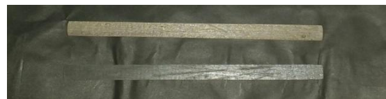
Figure 5: Compression test specimen with additives calcium silicate or silicon carbide.
