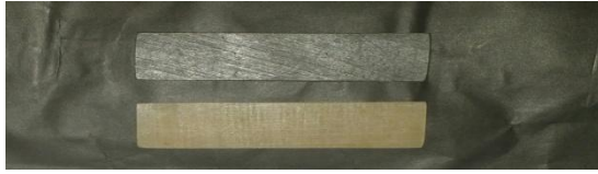
Figure 7: Bending test specimen with additives calcium silicate or silicon carbide.
