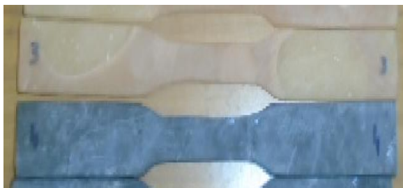
Figure 3: Tensile test specimen with additives calcium silicate or silicon carbide.
