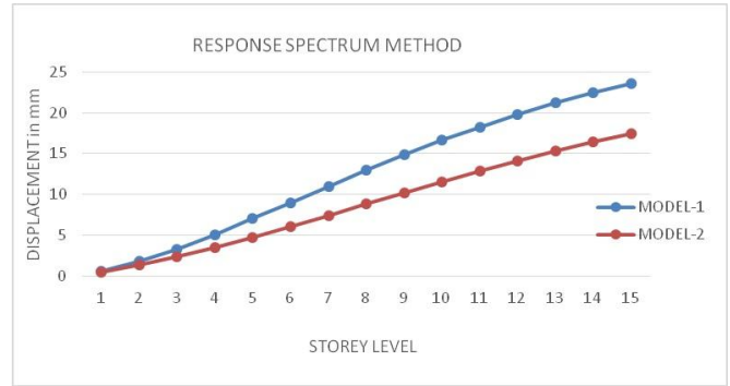
Fig.2: Comparison of model-1 and model-2 Storey displacements for response spectrum method
