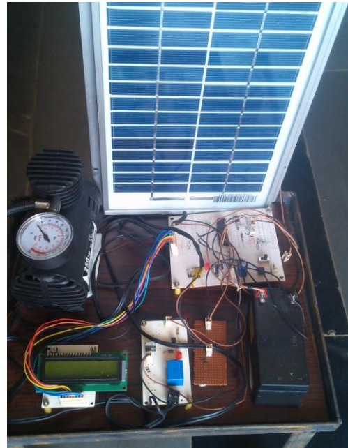
Fig 1.1: Working model of the solar based air compressor.
