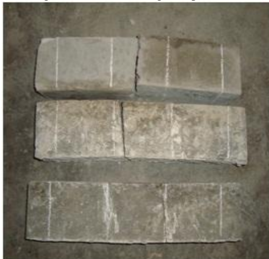
Figure 3.6: Flexural Failure Pattern
