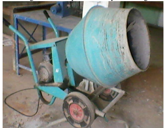
Figure 4. Concrete mixer used
