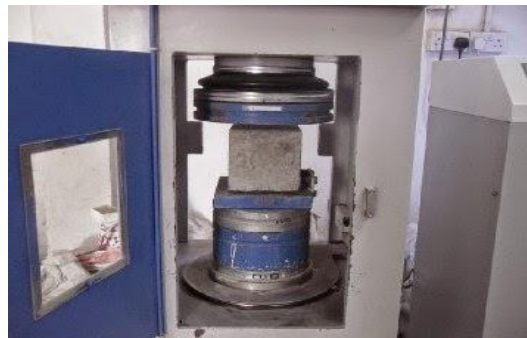
Figure 3. Compressive strength test setup
