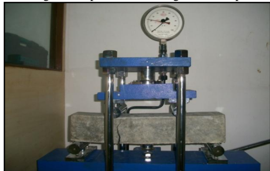
Figure 5. Flexural strength test setup
