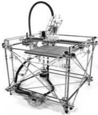
Figure 2. 6: Unmodified RapMan 3.0 from Bits for Bytes The VFDM extruder is designed to replace the original RapMan extruder with minimal changes. The standard RapMan heating system will be changed from a fixed resistance wire and fire cement configuration to a removable aluminium block which contains two power resistors. One of the power resistors is connected to the RapMan control board along with a thermistor for temperature control. The other power resistor is connected to an external circuit to enable a base heating load giving greater temperature control via the thermostat, see Figure 2.7.
