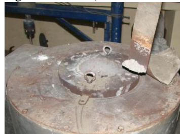
Fig. Removing the impurities – SLAG
