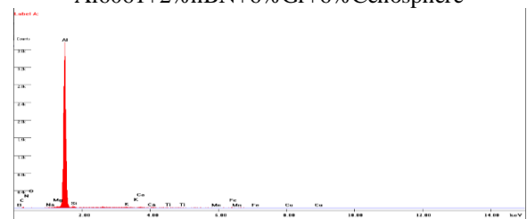
Fig.(d) EDS Analysis of Al6061+2%hBN+6%Gr+6% Cenosphere
