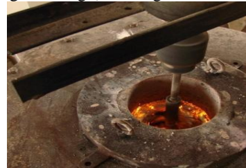
Fig. Stirring the Mixture (Matrix + Reinforcement)
