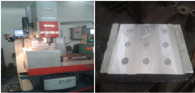
Figure:- 1.1 Experimental Setup Of Vertical CNC Drilling Machine & Final Image Of Work piece
