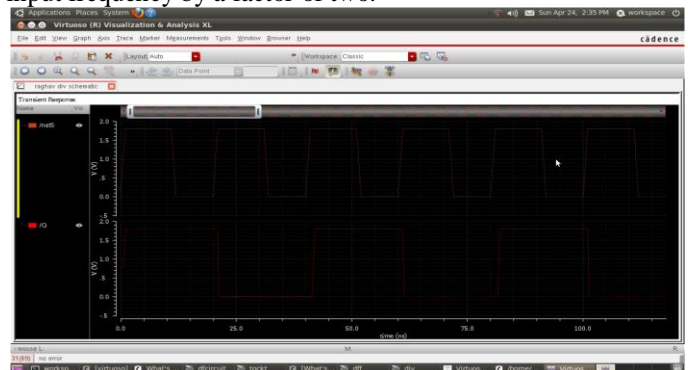
Fig 7.2: Output waveform of Frequency division by 2
