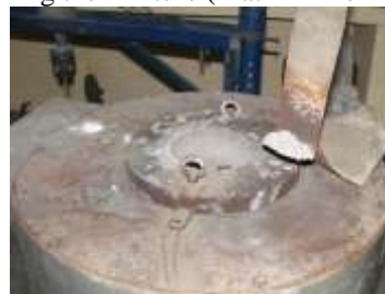
Fig.3 Removing the impurities – SLAG
