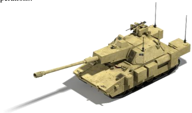
Figure 1: Non-Line of Sight Cannon (NLOS-C) The Reconnaissance and Surveillance Vehicle (RSV) consist of a set of advanced sensors technology which can able to detect, locate, track, classify and automatically identify targets from for-beyond ranges under all climatic conditions: day or night [14,15]. It includes a set of roof-mounted, long-range electro-optic infrared sensor, emitter mapping sensor
