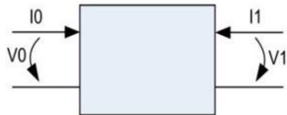
Fig. 1 A two-port network circuit with the indication of the current and voltage signals.
