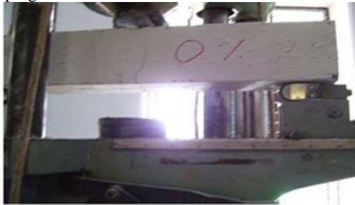
Fig. 3 Test Set Up for Beam
