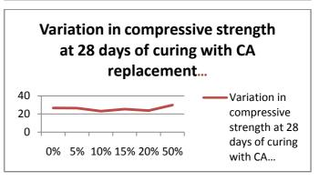
The above graphs shows the compressive strength of concrete containing marble chips. The strength increased with the increasing replacement of coarse aggregate up to 50%. The specimen with 50% marble chips showed 12.30% more compressive strength than the reference mix at 28-days.
