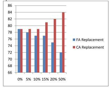
variation in slump (mm) with each level of aggregate
