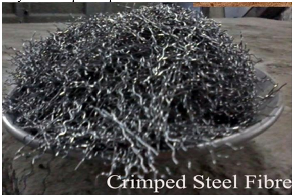
Figure 2.1 Crimped Steel Fibre
