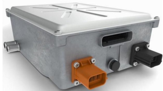
Fig. 4. The mechanical packaging of the charger. Waveforms of the input voltage, input current and PFC bus voltage of the charger are provided in Fig. 5 for the following test conditions: Vin = 240 V, Iin = 15 A, Po = 3300 W, Vo = 300 V, fsw = 70 kHz (PFC) and 200 kHz
