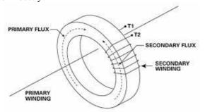
Like any transformer, a current transformer has a primary winding, a core and a secondary winding, although some transformers, including current transformers, use an air core. In principle, the only difference between a current
