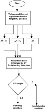
Fig-5 Flowchart for Flowchart for the proposed fuzzy rulebased scheme for islanding detection
