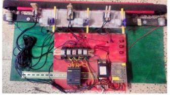
Above Fig. clearly shows that working of objects sorting system. A belt conveyor is used to feed the iron objects. It is driven by means of a the proximity sensors are use to sort the iron objects when actuated by the sensors. further the DC motor get activated and push the valve forward which push the iron object and sort the by height. Object such as boxes, packing load onto the conveyer belt. We are using for auto loader mechanism, then the different sizes objects moving toward the conveyer
