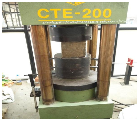
Figure 3: Compressive Test on Concrete
