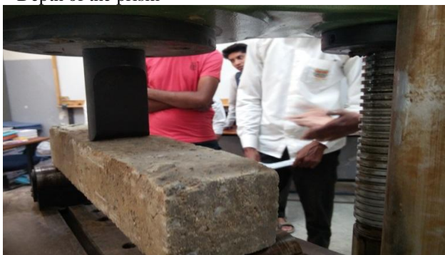
(Figure 4 : Flexural Test of Prism)
