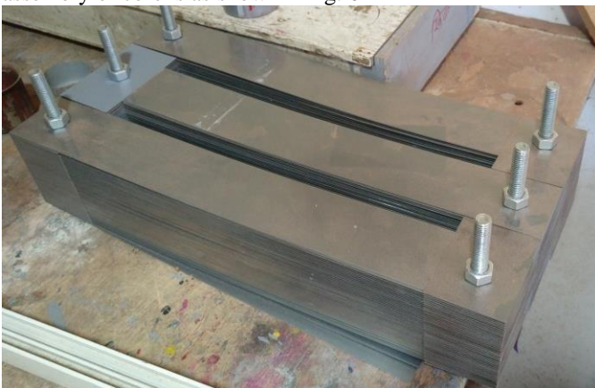
Figure 6: Core assembly of linear Autotransformer
