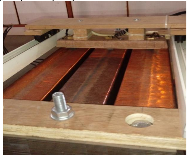
Figure 8: Brush holder and sliding mechanism
