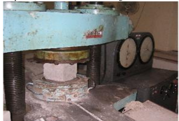
Fig.1. Details of cube testing under TOTM
