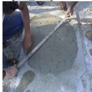
Fig.1.Abrams Slump flow Equipment
