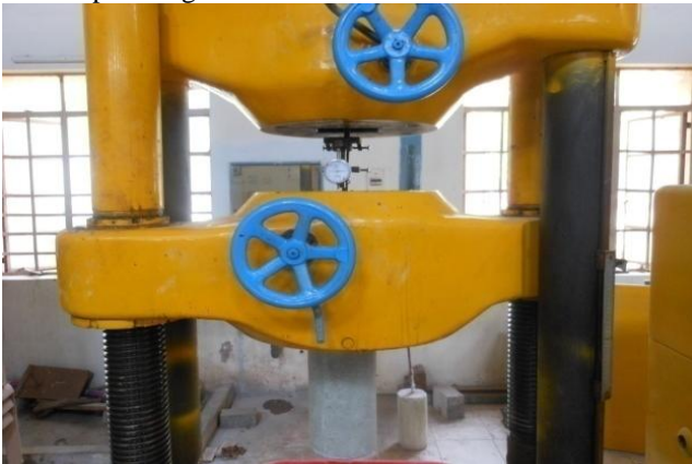
Fig.4. Details of the test setup for pull-out test.
