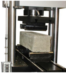
Fig no. 3: Flexural Strength Testing Arrangements
