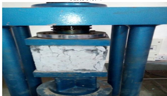
Compressive strength test
