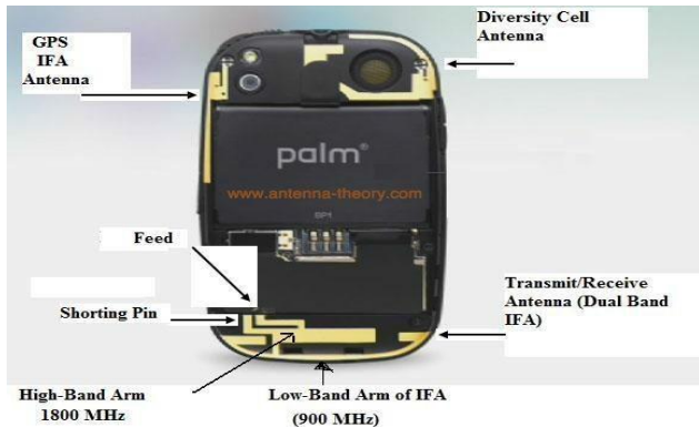
Figure Different Inverted F antennas fitted inside a mobile phone (Courtesy: www.antennatheory.com). inside a mobile phone for various applications.
