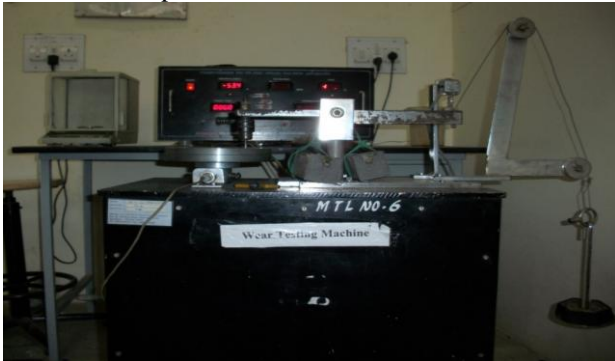
Fig.2 Pin-On-Disc wear testing machine
