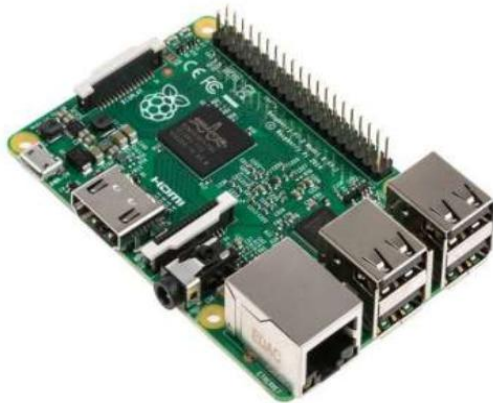
Figure 2: Shows the Raspberry Pi 2.
