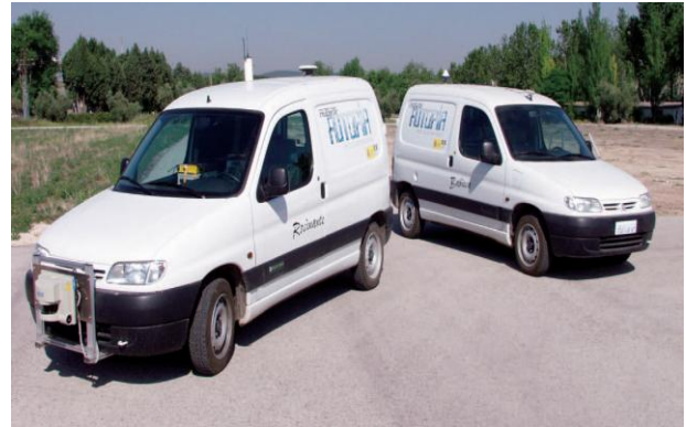
Figure 1. The AUTOPIA testbed vehicles. An embedded fuzzy-logic-based control system controls both speed and steering in each Citroën Berlingo.
