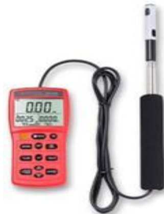
Figure 3.3: Hot Wire Anemometer
