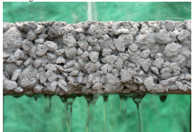
Fig 1: Infiltration of water through Pervious Concrete
