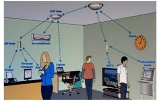
Here Li-Fi uses direct modulation without using intermediate frequencies. It uses small LEDs and photo detectors that is why it is possible to create small, low-complex transceiver units that enables any LED light to act as high speed data transmitter. Big Data is a high volume, high velocity and high variety information assets that demands cost-effective
