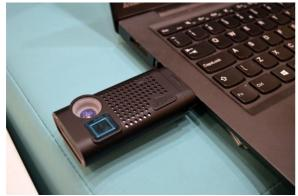
Recently, this device LiFi-x is invented by PureLiFi Company which provides 40Mbps downlink and upward link communication. Which is the world's fastest, smallest and most secure Li-Fi system. Li-Fi is emerging technology in the field of Internet of Things and the applications and advancement is beyond the imagination.
