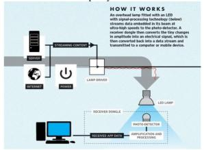
electricity is controlled due to this LED blinks, when power is applied then LED is ON so it gives bit 1 and for OFF condition of LED it shows 0 bit. Due to this rapid ON and OFF conditions LEDs are most suitable for this data transmission in addition to that LED provides illumination and transmission at low cost. Finally decoded data is transferred to destination device.
