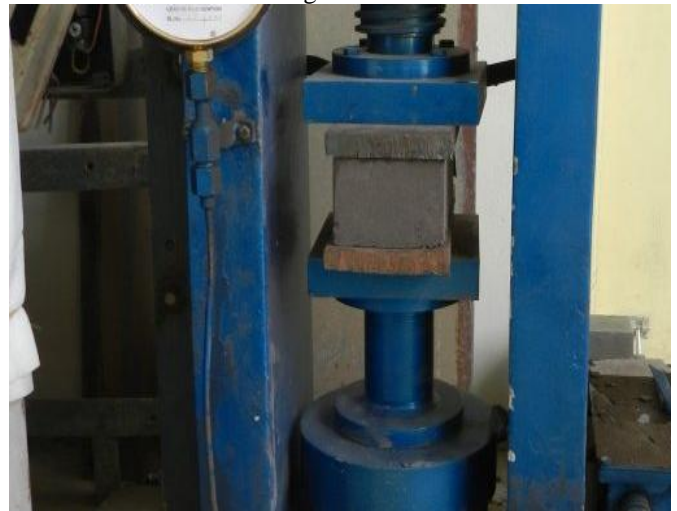
Figure4: Placing of concrete cube specimen in Compression testing machine.
