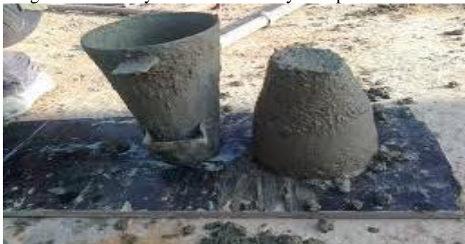
Fig 3: Workability test of concrete by slump cone method
