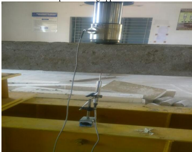
Figure 5: Flexural strength test of Beam specimen on centre point loading apparatus.
