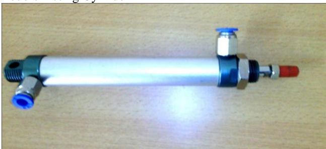
120psi Pneumatic double acting cylinder(60*80)
