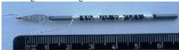
Figure 10. Showing a micro-tube with the Ni mesh inserted
