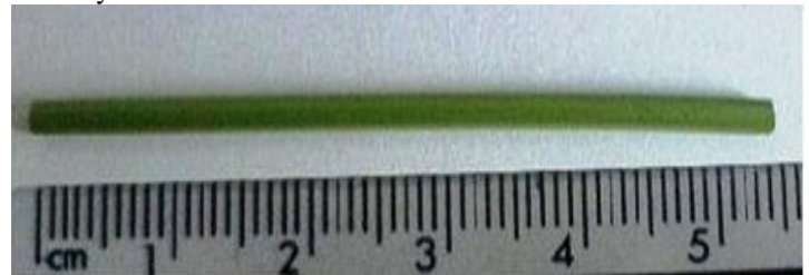
Figure 3 Image of the NiO/YSZ tube supplied by Adaptive Materials Inc
