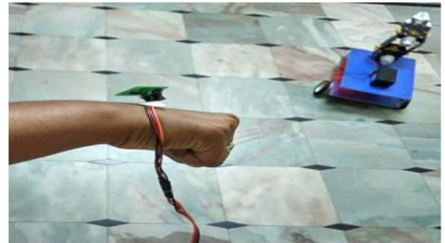
Fig 7: MEMS used to move Robot in Left Direction
