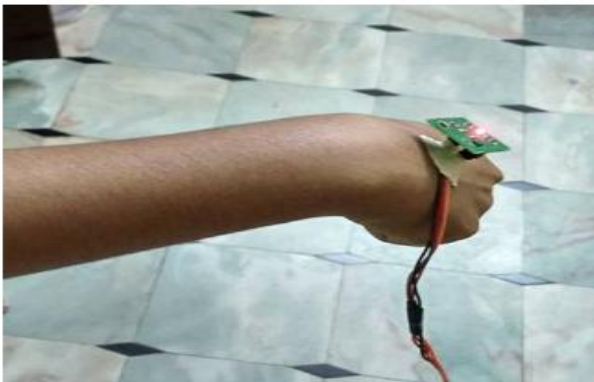
Fig 5: MEMS used to move Robot in Forward direction
